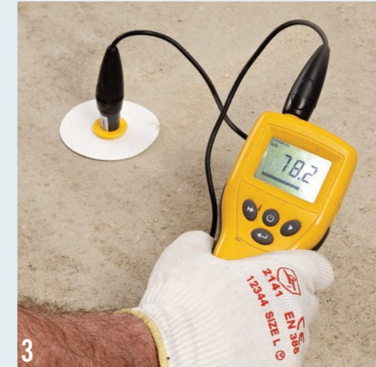
3 Insert the humidity probe. Readings above 75% RH require treatment.
