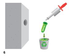
Expel the RivePipe from the RiveOut performing the counterweight action again, but now, in the opposite direction to the extraction. Keep the Rivepipe for your next reuse. The formwork tie hole remains now clean and homogeneous, and prepared to be sealed with RiveStop.
