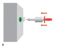
Once the wall has been formed, and the panels have been released from their framing, insert the RiveOut extraction tool's tip into the RivePipe. Screw the RiveOut head clockwise into the Rivepipe.
