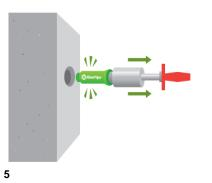
Remove the RivePipe with the help of the RiveOut by performing a counterweight action, with a linear displacement, in the direction from the wall towards the operator. This action must be done on both sides of the wall, in order to extract the two parts: female and male.
