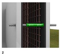
Place the RivePipe between the formwork panels to protect the tie rods.
