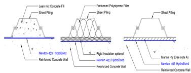
The adjacent drawings show examples of facing off secant and sheet piling ready for the application of 403 HydroBond. The same detailing applies for 402 CSS-M.
