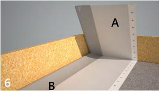
At internal corners, make a crease at the change in direction. Once the crease is formed, lift up the flap marked A and invert the upstand marked B so that the upstand of the flap A is in front of the main sheet upstand as shown in Fig. 7.
