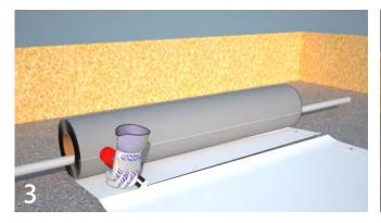
Measure the perimeter of the formwork to determine the length of the membrane required. Make provision for 70mm overlaps to each end joint of the 20m long membrane rolls. When cutting the membrane use a retractable craft knife or sharp shears whilst wearing safety gloves.
