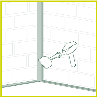
Form chase at wall to floor and all internal wall angles minimum 10mm x 10mm.
